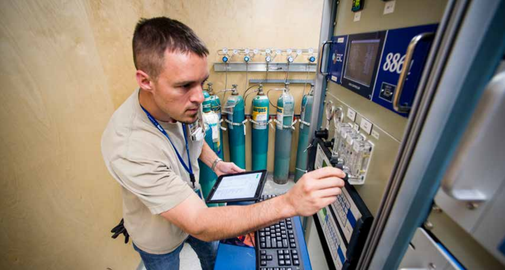
Nathan Pickrell, an Environmental Instrument Technician, inspects the Continuous Emissions Monitoring System at Spurlock Station.
